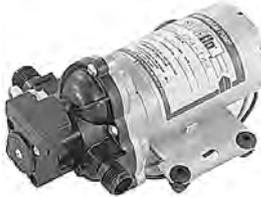
This pump is a lighter duty pump than the 145/534. It will turn on at 28 PSI and off at 40 PSI. It can be used without a pressure tank, coming on when the faucet is on and shutting off when the faucet is turned off. However, we always recommend the use of even
